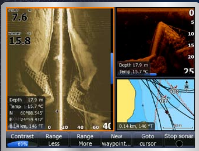
TrackBack™: Scroll back simultaneously through sonar history and chartplotter trail from sonar or StructureScan™ display to easily mark waypoints, and continue to record data while reviewing history.
