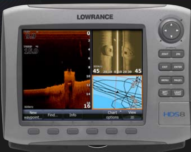
TrackBack™: Scroll back simultaneously through sonar history and chartplotter trail from sonar or StructureScan™ display to easily mark waypoints, and continue to record data while reviewing history.
